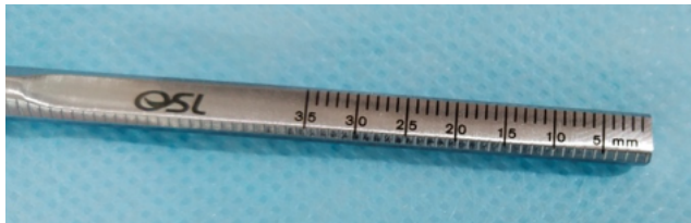
Fig. 2: Scale with mirror recording upto 35 mm
