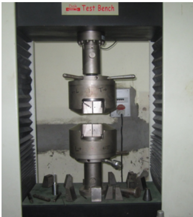
Fig. 4: Universal testing machine (Dak Systems Inc.'s Series 9000)
