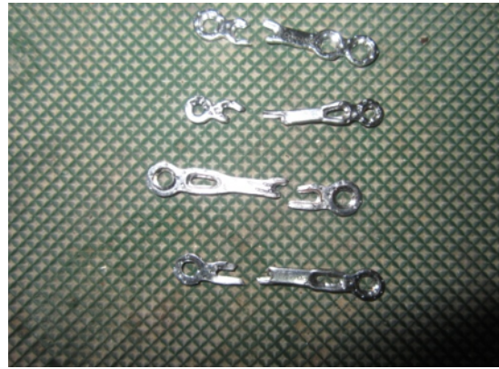
Fig. 5: Miniplates tested for tensile strength.
