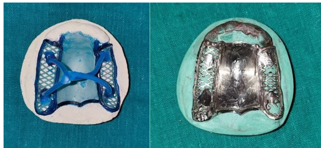
Figure 6: Wax pattern with sprue attached for base metal casting
